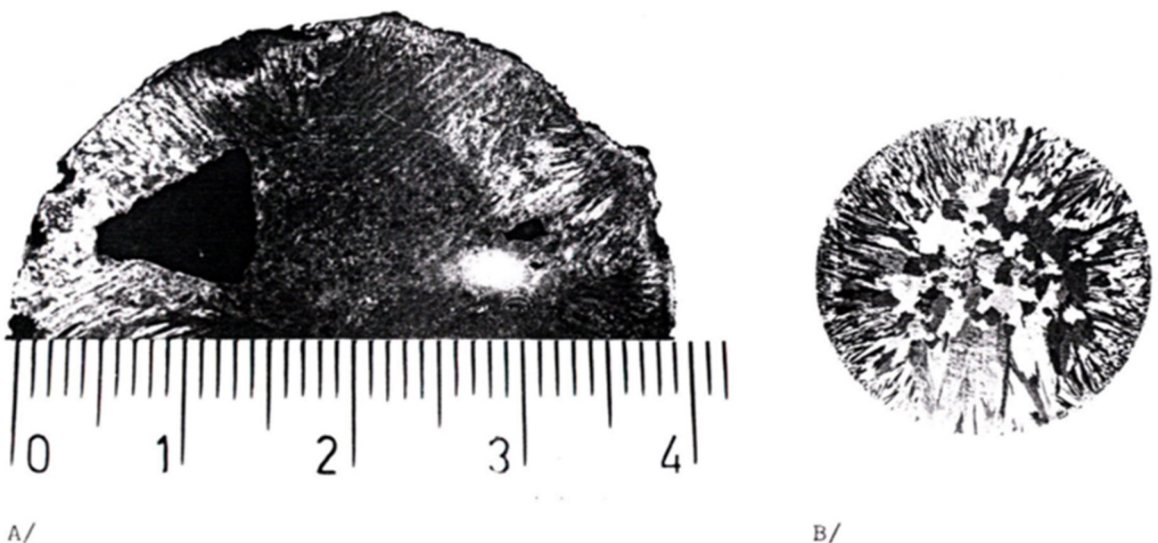
Fig.1. Macrostructure of the Cu-Cr-Ni-Si alloy A) Too short time or too low melting temperature (large undissolved pieces of chromium visible) B) Optimal melting time and temperature (structure after etching)
