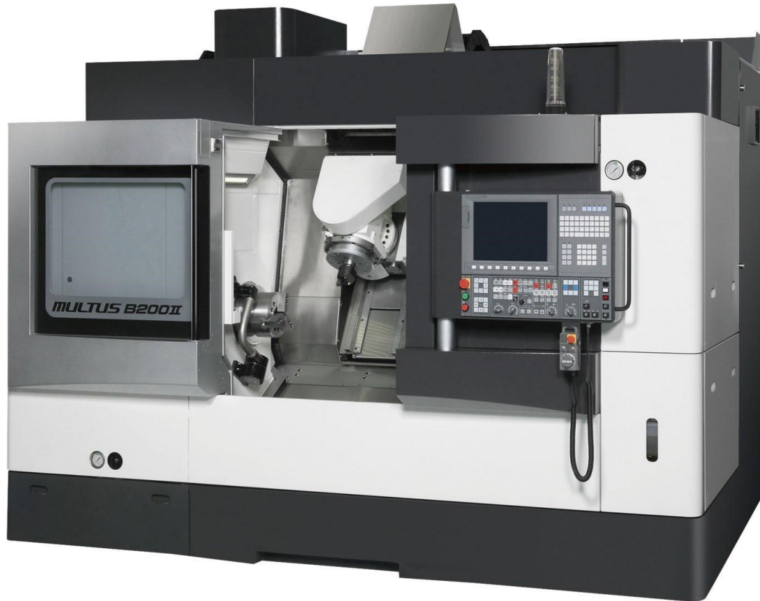
Figure 4. Multitasking machining center OKUMA MULTUS B200II at Technopark Gliwice.
