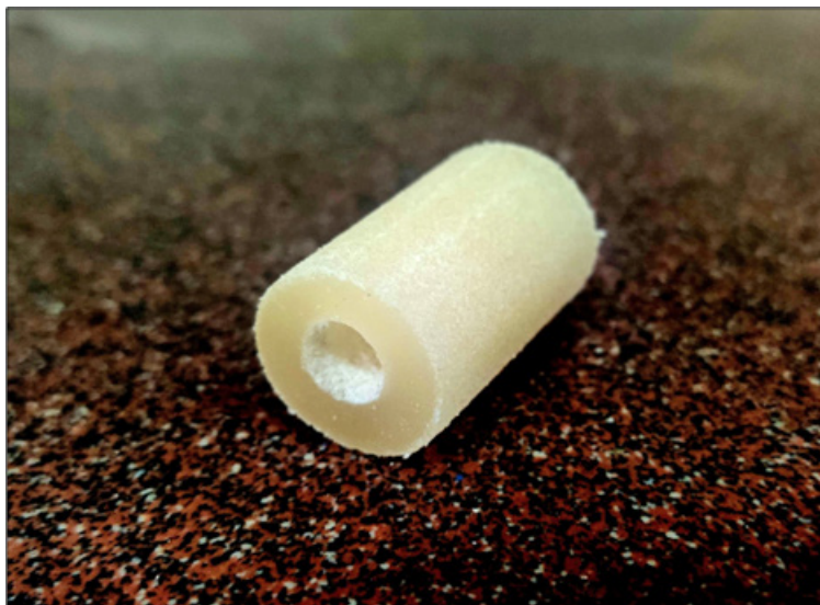
Figure 5. Cylindrical charge prepared for the burning test
