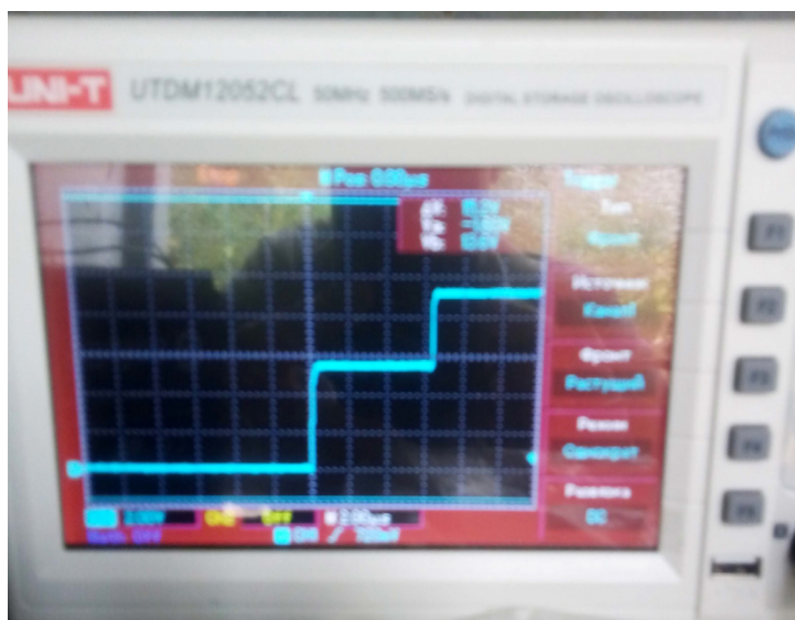
Figure 4. An oscillogram obtained from the shorting of a pair of contact sensors with a shaped-charge jet
