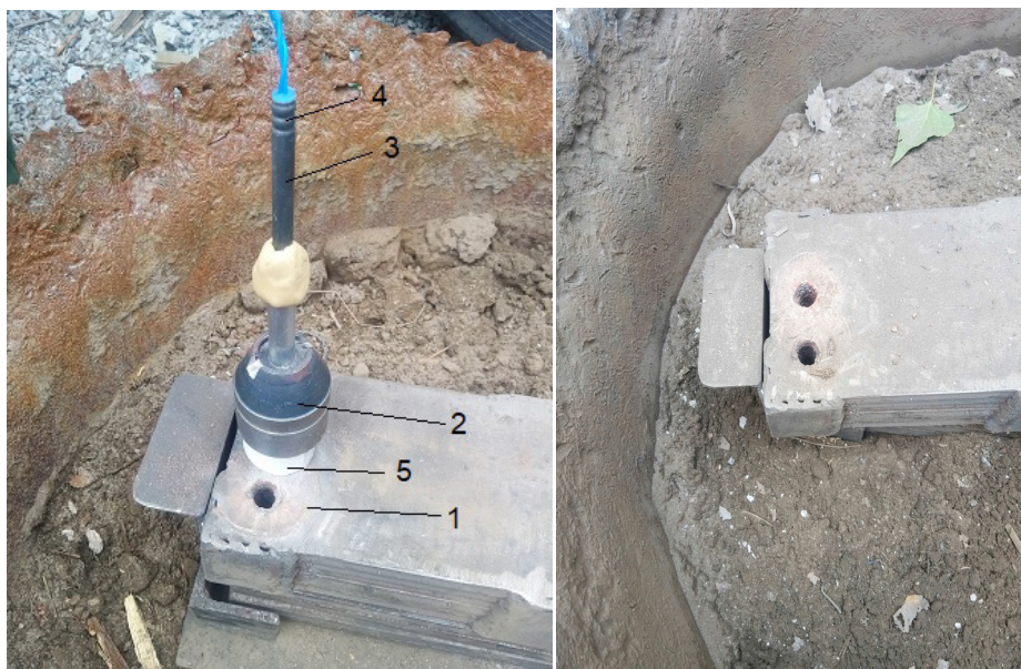
Figure 3. General view of the experimental set-up (left) and the target after the shot (right): 1 – target, 2 – charge, 3 – detonating cord, 4 – electric detonator and 5 – plastic cylinder
