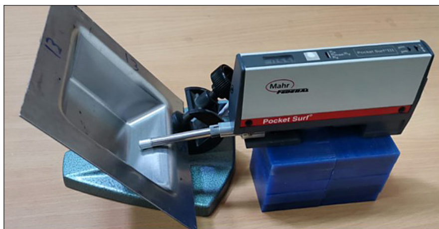
Fig. 7. The measurement process of the surface roughness
