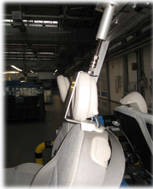
Fig. 1. Measurement of the friction of the head restraint ejecting.
