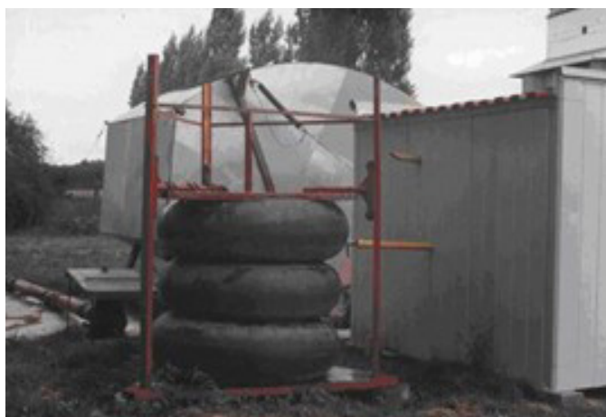
Fig. 7. Prototype of the biogas reservoir, consisting of flexible rings [archive of the Institute]
