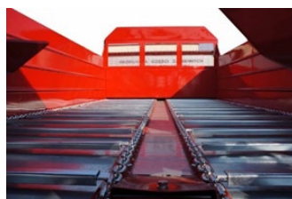
Fig. 4. Bulk trailer with a floor and slat conveyor Source: author's own photograph
