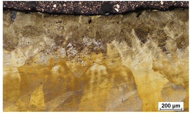
Fig. 9. Microphotograph showing Hadfield steel after solution heat treatment
