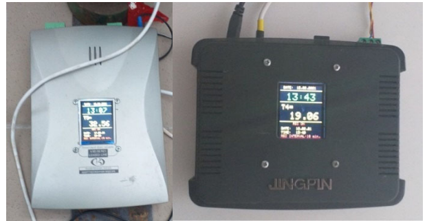
Fig. 3. Secondary devices for continuous monitoring of temperature values of the experimental stand
