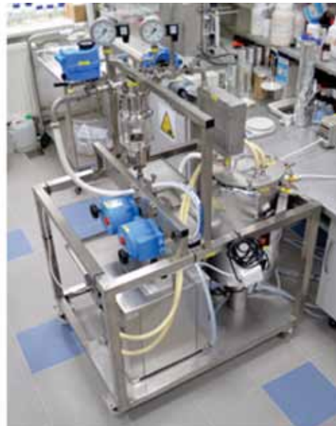
Fig. 1. Pre-filtration stand for testing filtration and separation properties of non-woven depth filters: (a) 3D scheme of the stand construction, (b) built prototype stand before automation
