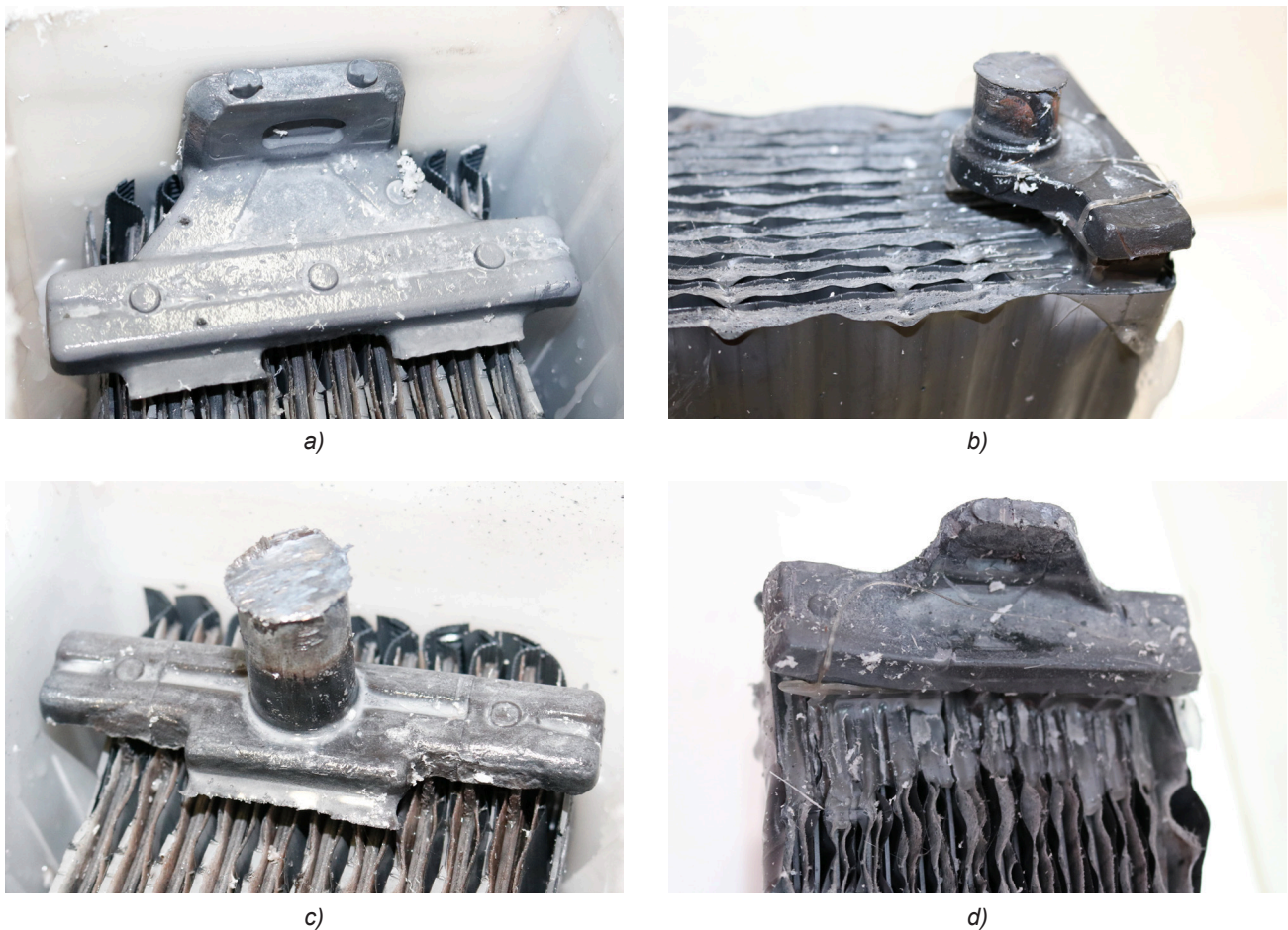
Fig. 3. The cast-on-strap positive and negative joints of a lead acid battery [photo E. Jankowska]
