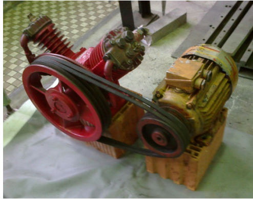
Fig. 1. General view of the Espholin H3S piston compressor assembly before mounting on the foundation
