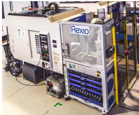
Figure 1. Robotic pallet system (illustrative example), source Metal Team advertising materials.
