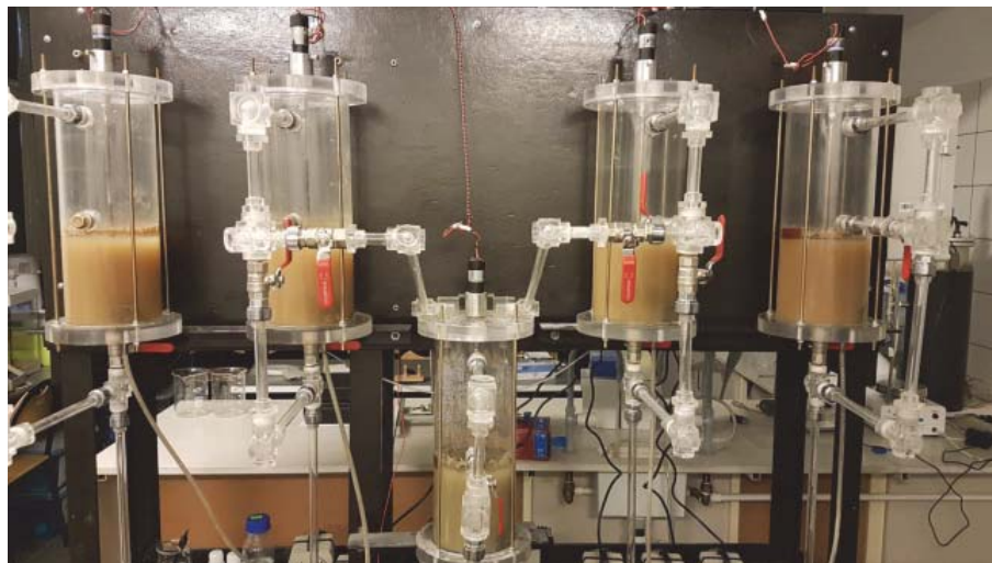
Fig. 1. Four batch reactors used in the presented studies (the 5-th reactor at the bottom is used as a reservoir for biomass)
