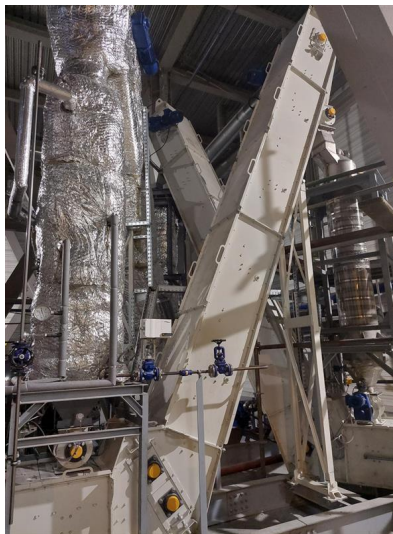
Figure 1: The test stand scheme (a) and photo (b): 1 – feeder, 2 – reactor, 3 – flue gas cooler, 4 – conveyor belts, 5 – heat exchanger intended for heat recovery, 6 – heat exchangers.
