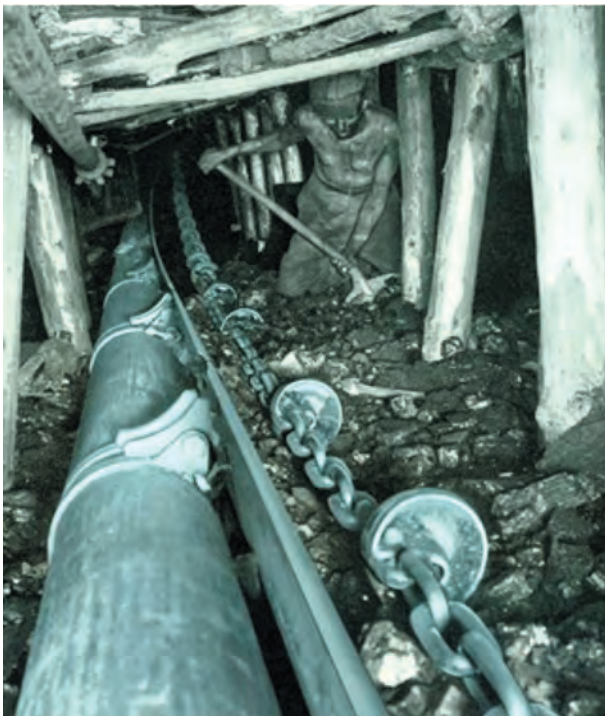
Fig. 2. Retarding disc conveyor
