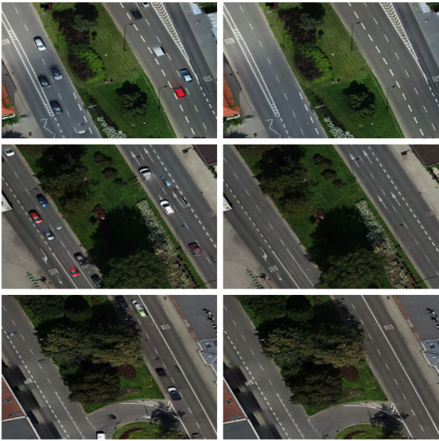
Figure 11. Comparison of the orthophotomaps generated without automatic masking (left) and with automatic masking (right)
