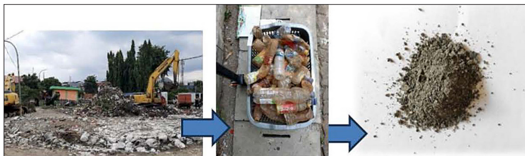
Figure 3. Processing step of PET charcoal powder material from river debris
