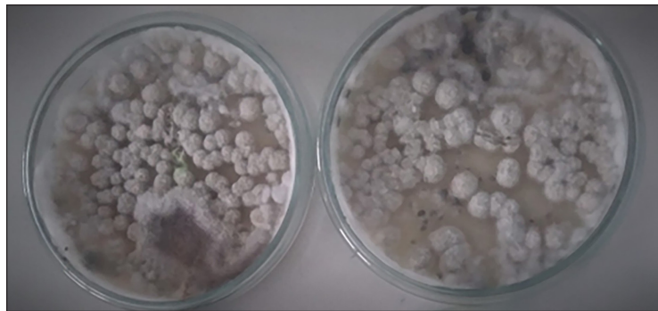
Figure 11. Swab method: HL-5C composite – after 1 month, the predominance of the genus Absidia sp.
