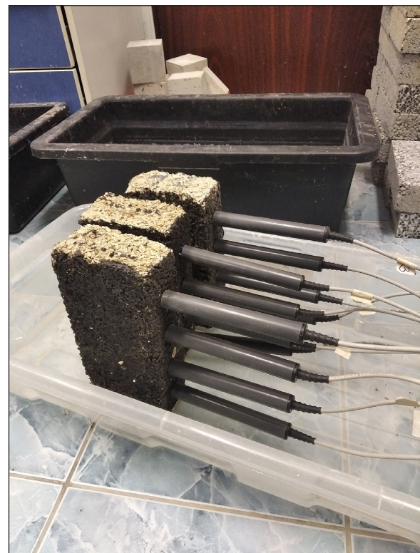
Figure 3. General view of the sample during capillary rise test
