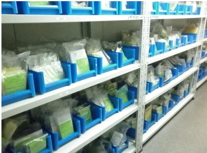
Fig. 1. Typical aviation warehouse of small products stored in plastic bags and containers, away from windows and sources of heat. Green warehouse tags confirm that the products are within their expiry date
