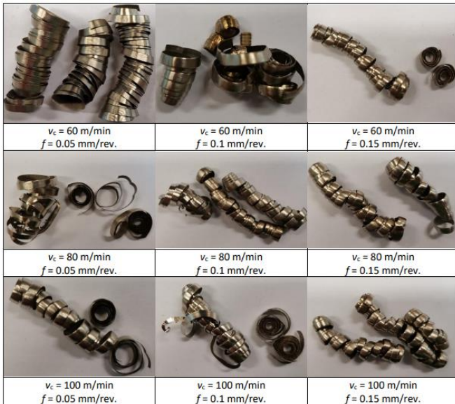
Fig. 12. Chip evaluation as a function of cutting speed and feed rate
