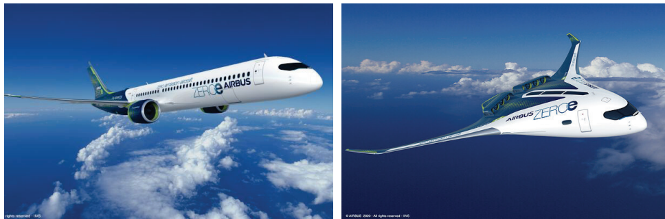
Fig. 1. Artist's impression of hydrogen-powered commercial aircraft envisioned by AIRBUS. On the left is a plane with two hydrogen turbofan engines providing thrust. The liquid hydrogen storage and distribution system are located behind the rear pressure bulkhead. On the right is a Blended-Wing Body aircraft with much optional storage of LH 2 and powered by hybrid-hydrogen turbofan engines.
