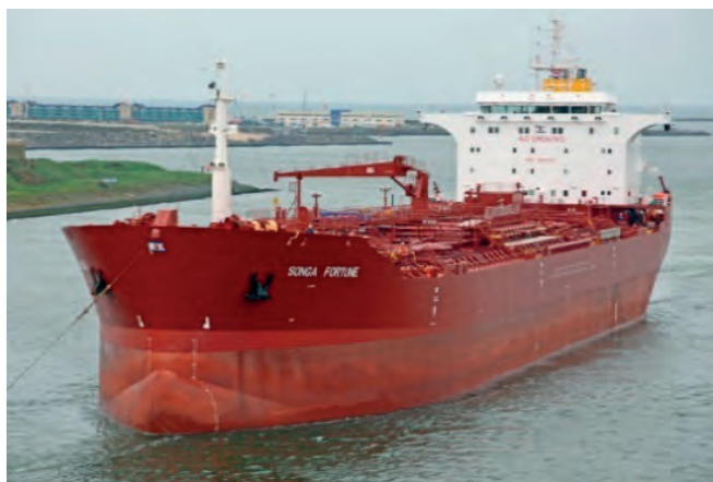
Fig. 4. Tanker with deadweight of 45,500 t with a MAN 6S50ME-B9.3 main engine
