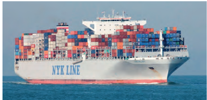
Fig. 6. Container ship with deadweight of 122,000 t and a MAN 12S90ME-C9.2 main engine
