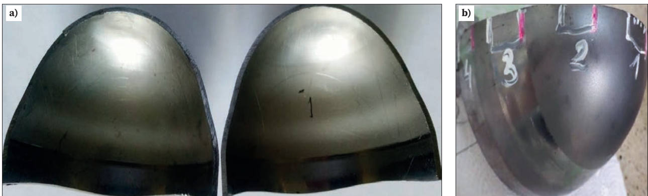
Fig. 2. Liner drawpieces cut along the main stamping axis (a) and sampling diagram (b)
