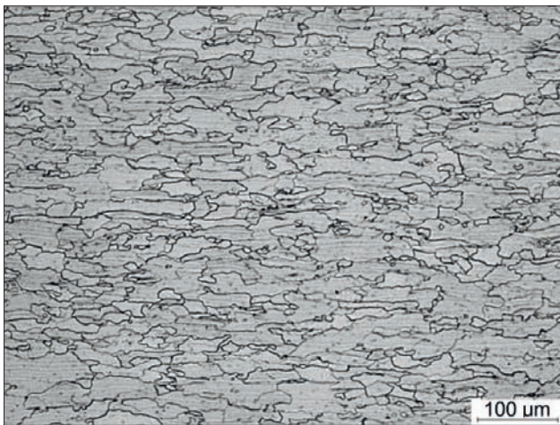
Fig. 10. Microstructure of 04J steel sheets occurring in the direction transverse to the rolling direction, magn. 100× and 400×
