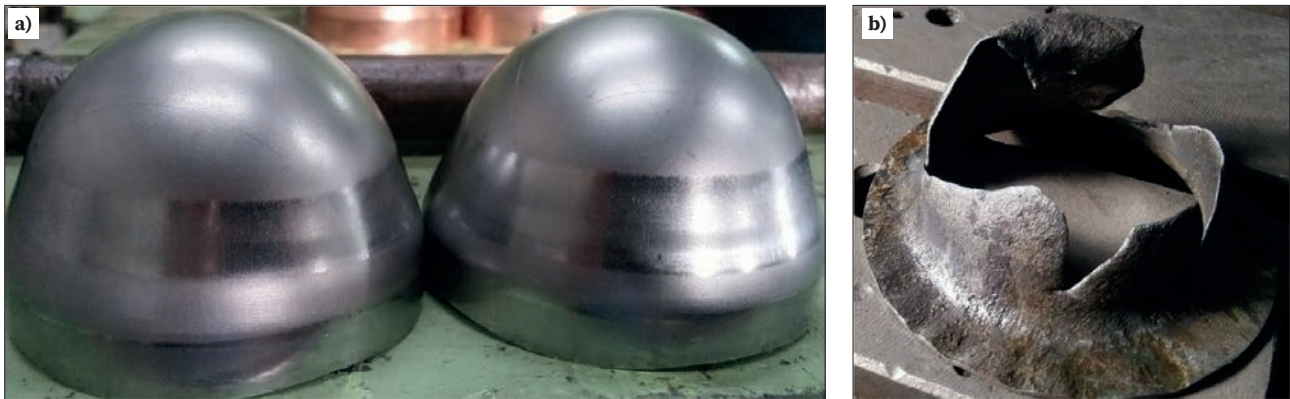
Fig. 1. Photographs of correct liner drawpieces made of DC04 and 04J steel (a) and of defective drawpiece made of 004G steel (b)
