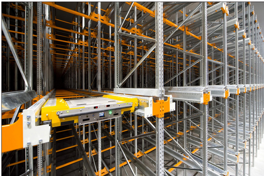
Figure 3. AutoMAG Shuttle semi-automatic dense storage system – a proprietary system by PROMAG S.A. [20]
