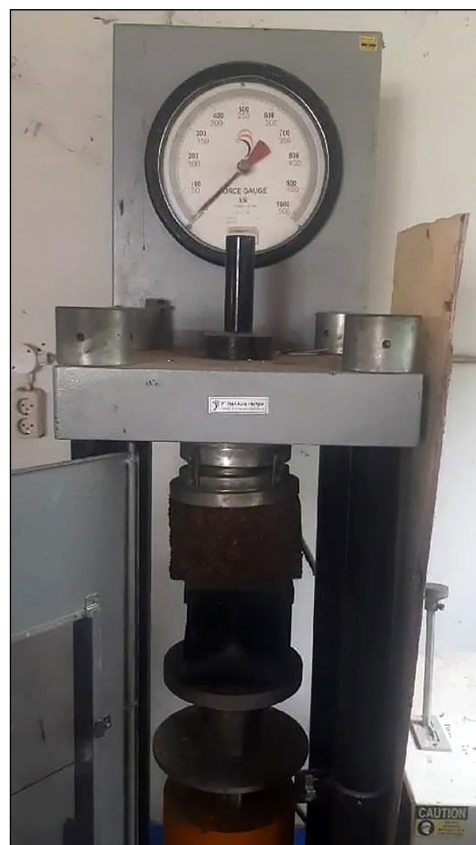
Figure 6. Measurement of compressive strength of briquettes
