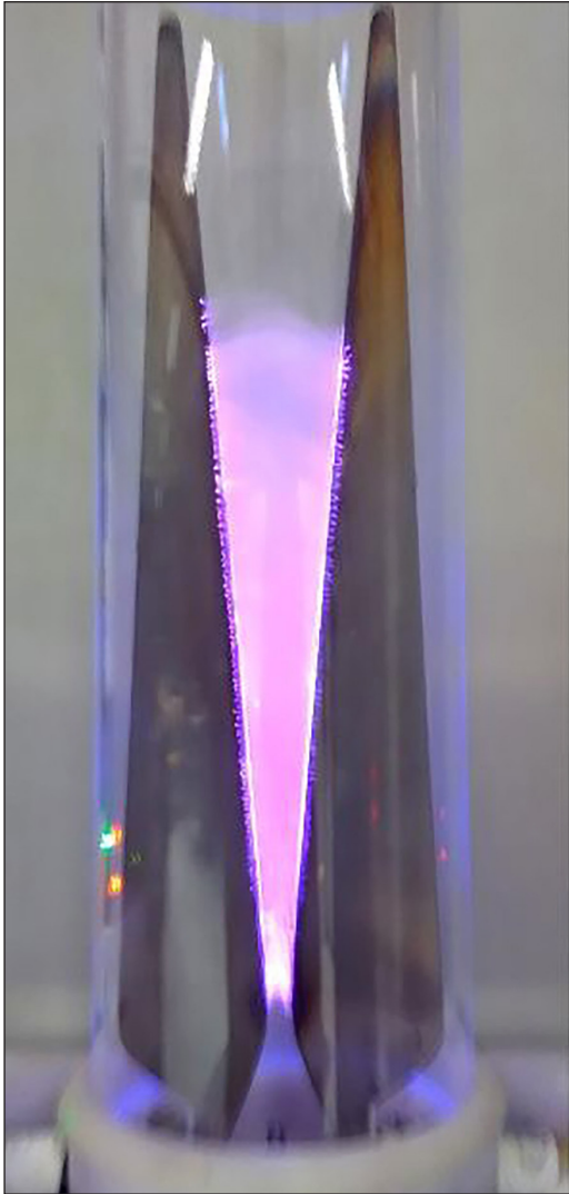
Figure 3. Double electrode GlidArc-type plasma reactor which has an adjustable inter-electrode spacing – regular photo [16]
