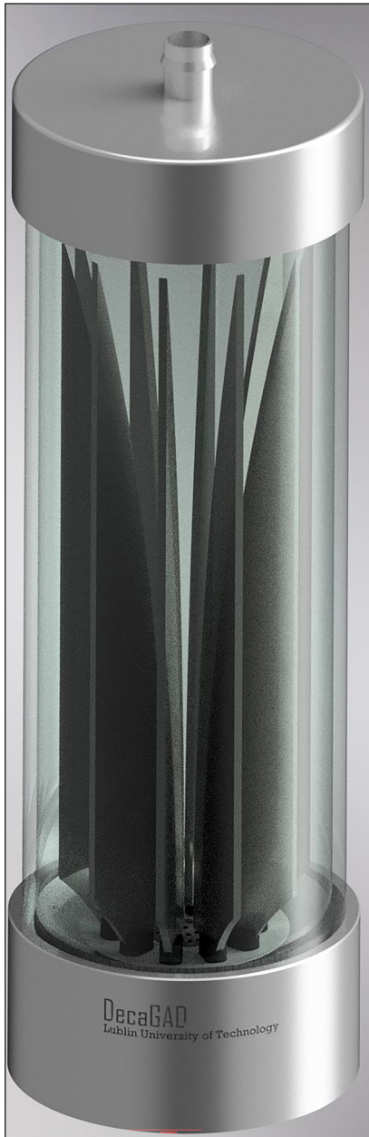
Figure 17. The render of DecaGAD Plasma reactor obtained in Autodesk Inventor Studio environment
