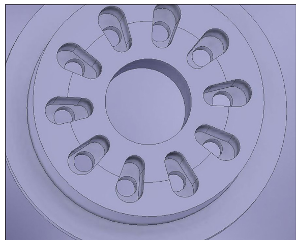
Figure 11. Electrode holder with holes made for inserting ten electrodes, obtained using a circular pattern tool (circular pattern)
