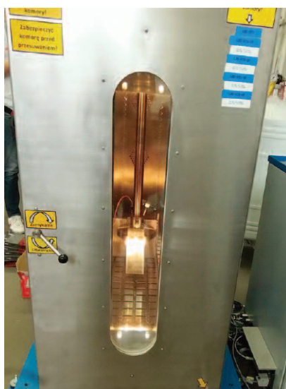
Photo 2. A endurance testing machine integrated with a temperature chamber
