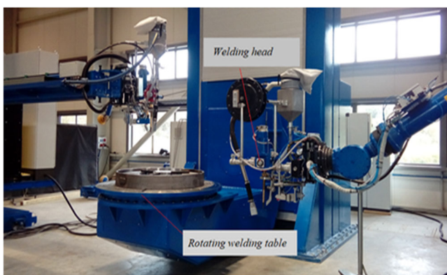
Fig. 1. FANUC-Robot M900iA submerged arc welding station
