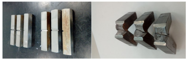
Fig. 8. Samples S355JR t=25 before and after the impact test. The specimens show V notches in the weld axis (VWT) and in the heat affected zone (VHT)
