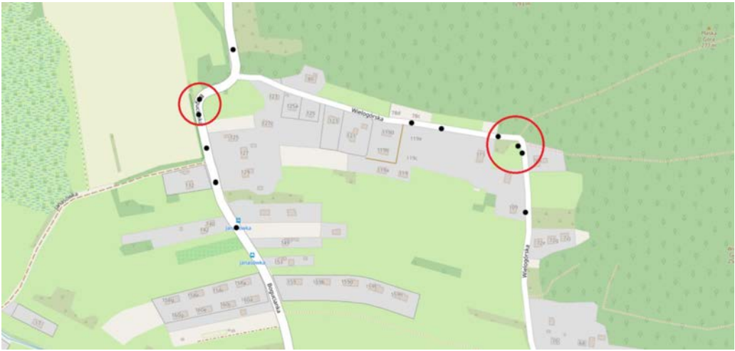
Figure 8. Closely located points in the irregular grid that can be merged into one point (base map: map data copyrighted OpenStreetMap contributors and available from https://www.openstreetmap.org )
