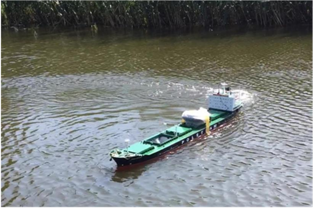
Fig. 6 Ship's model during circulation investigations [4,11]
