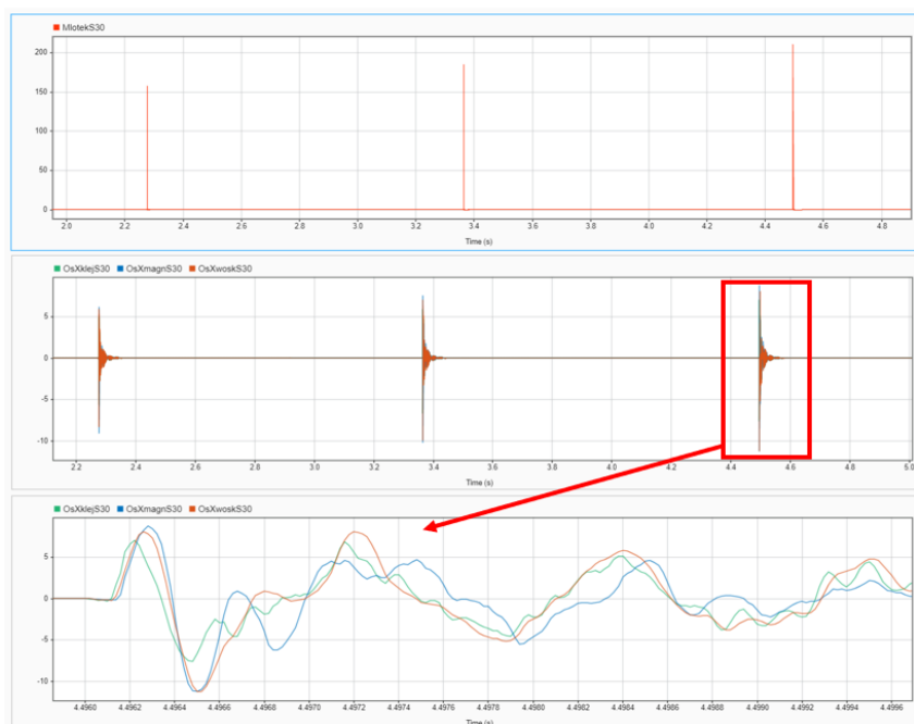
Fig. 9. The trace of the recorded vibration signals and the inductor signal shown in the MatLab software; X-axis-excitation with a medium tip of a modal hammer. From the top: inductor signal, time trace of sensors. Description of the markings: green - glue, blue - magnet, orange - wax
