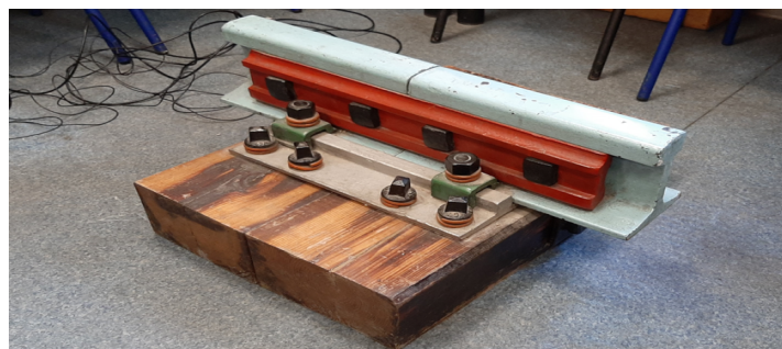
Fig. 4. Test stand – model of railroad used on sleeper beams
