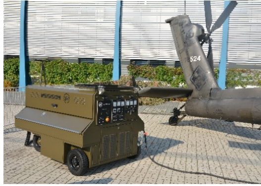
Fig. 4. Electrical power unit LUZES II/M
