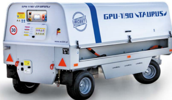
Fig. 5. Electrical power unit GPU-7/90 TAURUS
