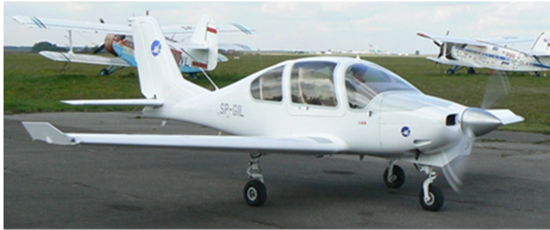
Fig. 1. The I-23 Manager driven by a low-power piston engine and a 2-blade propeller.
