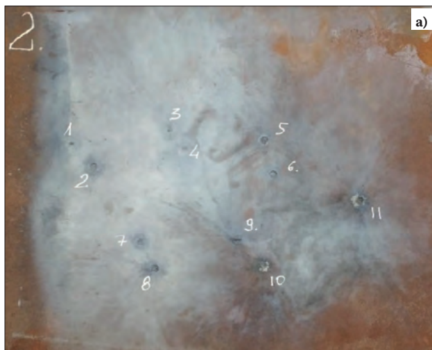
Fig. 29. Plates after firing. a) heat P2, thickness 8.0 mm; b) heat P1, thickness 7.0 mm
