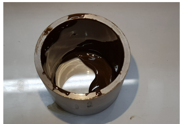
Fig. 5. Bushing with layer of oil mud inside
