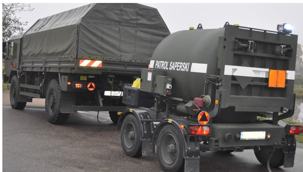
Figure 4. A vehicle and the Wiktoria ventilated container for transporting explosives mounted on a trailer [9]
