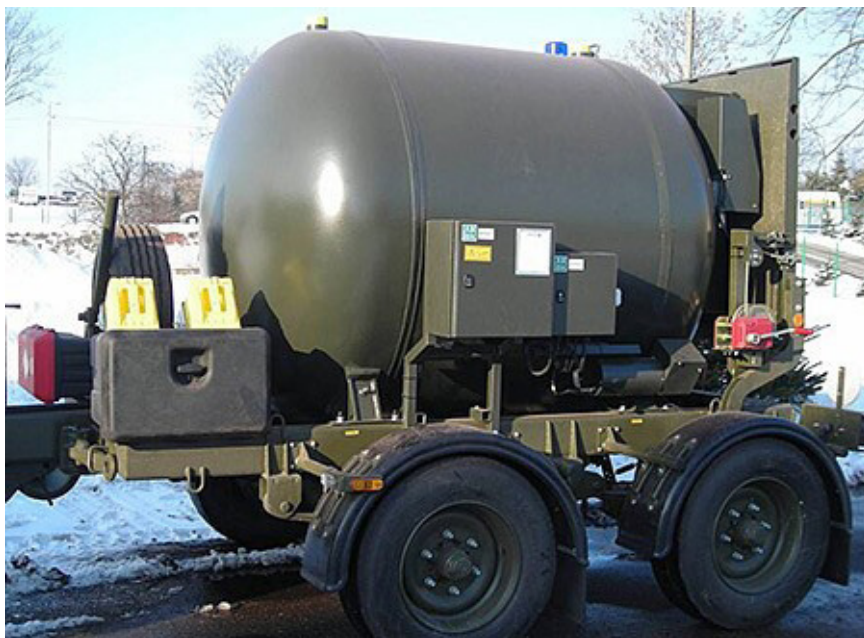
Figure 3. The Wiktoria ventilated container for transporting explosives on a trailer [11]
