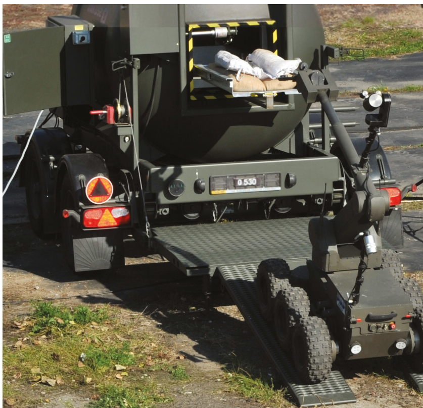
Figure 7. The Wiktoria ventilated container for transporting explosives [11]
