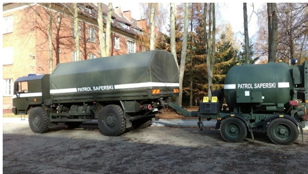
Figure 2. A sapper vehicle with the Wiktoria ventilated container for transporting explosives mounted on a trailer [9]
