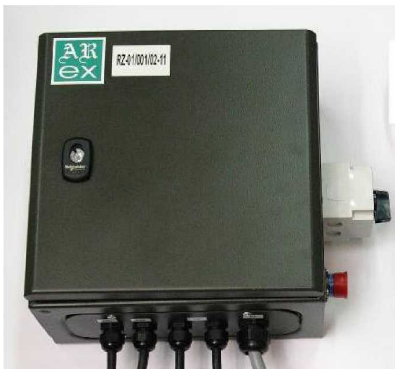
Figure 6. A view of the PSV-01 control panel and the RZ-1 control unit (Source: Arex archive)
