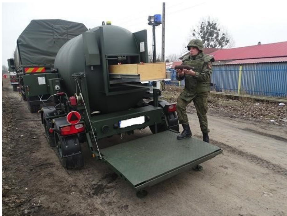
Figure 5. The Wiktoria ventilated container for transporting explosives on a trailer [9]
