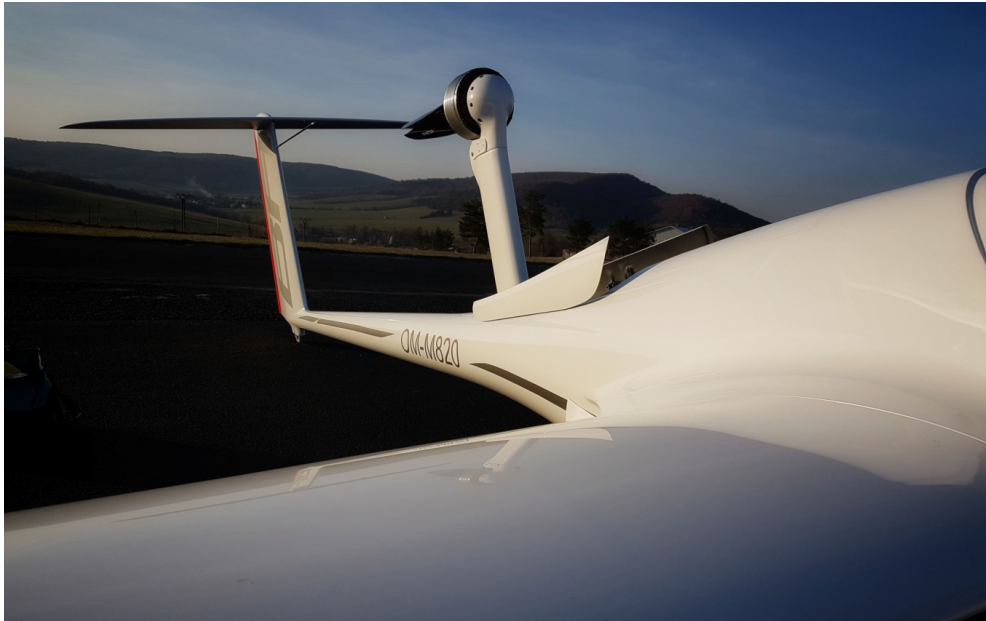
Fig. 5. The electric motor glider GP14 SE, produced by Peszke S.C. company [10]
