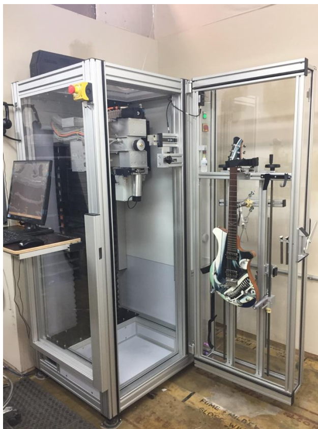
Fig. 3. A CNC machine used to make sure all the frets of the guitar are at their optimal place on a guitar neck. [ https://facfox.com/docs/kb/cnc-machining-for-musical-instruments-how-technology-enhances-artistry ]
