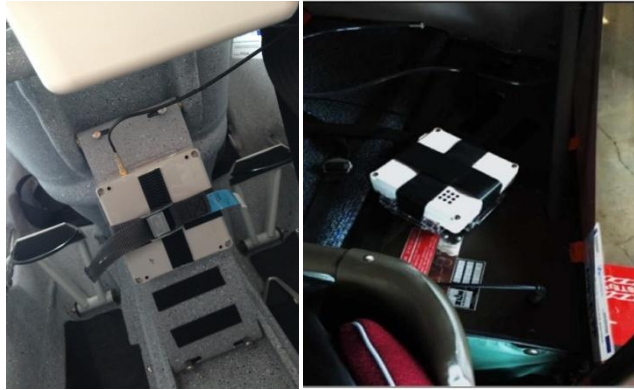
Fig. 3 Portable ASSD+PL modules fitted in the aircraft (MDM-1 FOX glider, ZLIN 242 airplane)
