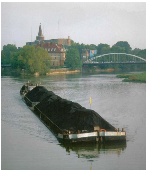
Fig. 7. Push train of deck barges on the Oder.
