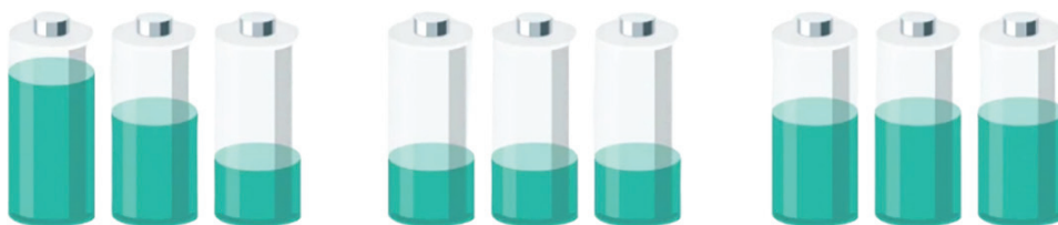
Figure 1. Battery pack from left to right: without balancing, with passive balancing, with active balancing.
