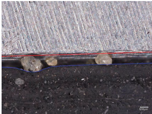
Fig. 12. Contact surface of the steel-NBR pair, with solid particles of mineral origin between them, showing the local deformation of the flexible NBR.
