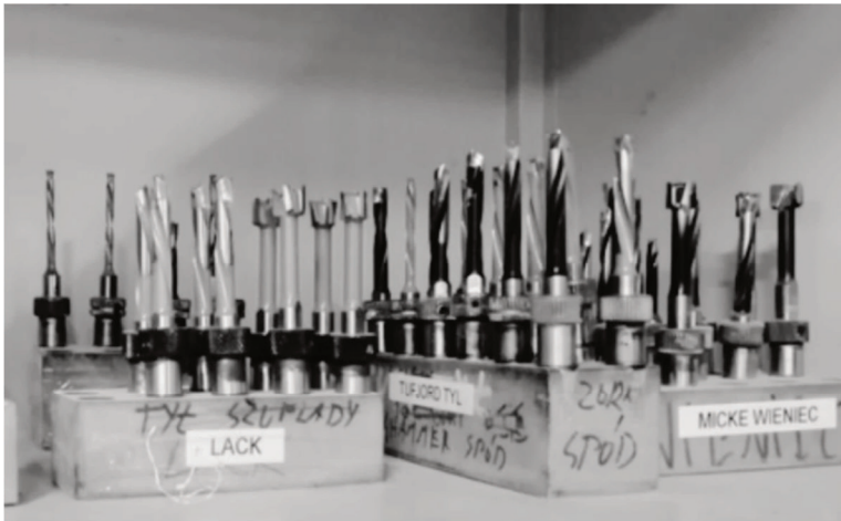
Fig. 7. Way of storing drill bits before introducing a change (authors' own development)
