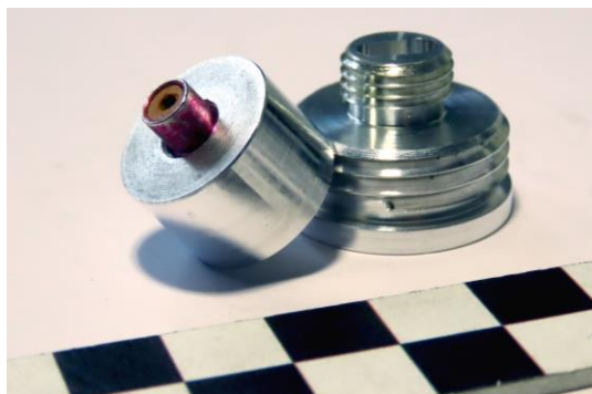
Fig. 2. Initiating system for the igniter of rocket projectile: 1) fitting of the booster charge, 2) booster charge in the fitting, 3) fitting of ignition primers, 4) electric ignition primer, 5) electric wires of the primer
