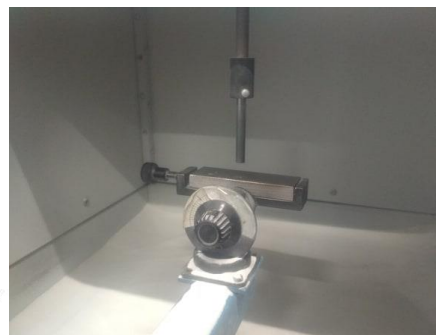
Fig. 3 Scheme [23] and a picture of the erosive test stand
