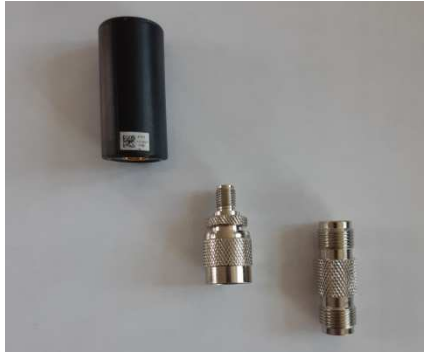
Figure 2. Antenna M1575HCT-22P and transition connector. Source: authors' photo.
