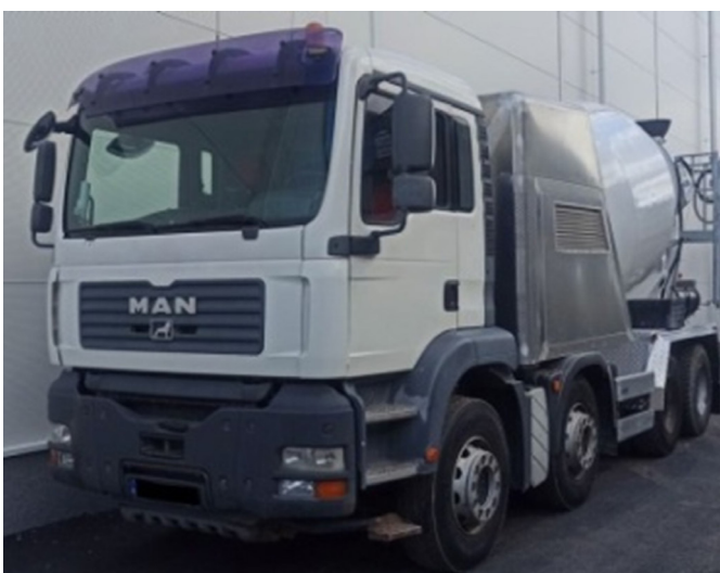
Fig. 6. Vehicle for operational testing of an innovative self-built mixer body work
