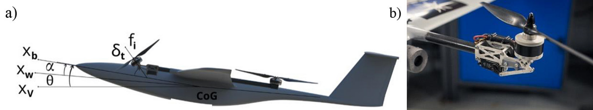
Figure 2. Transition mode: a) front-rear rotors configuration (where: CoG – centre of gravity, \delta_t – deflection of the rotor nacelle, f_i – i -th rotor force ( i = 1, \dots, 4 ), \alpha – angle of attack, \theta – pitch angle, x_b – coordinate x in the body reference frame, x_w – coordinate x in the wind reference frame, x_v – coordinate x in the inertial reference frame with the origin in the CoG), b) tilt mechanism
