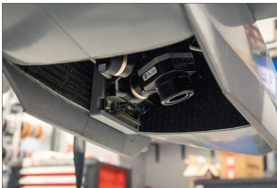
Figure 3. Cargo compartment with thermal imaging module
